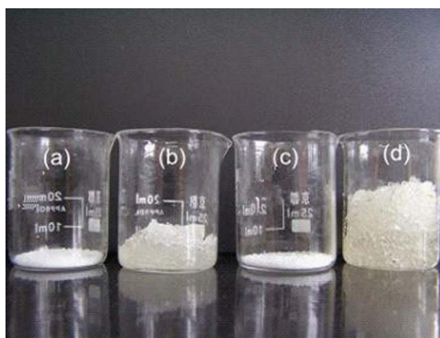
Figure 4. Swelling curve of A4 and B17: (a) dried B17, (b) wet B17 swollen in dichloromethane for 24 h, (c) dried A4, and (d) wet A4 swollen in dichloromethane for 24 h. [Color figure can be viewed in the online issue, which is available at wileyonlinelibrary.com .]
